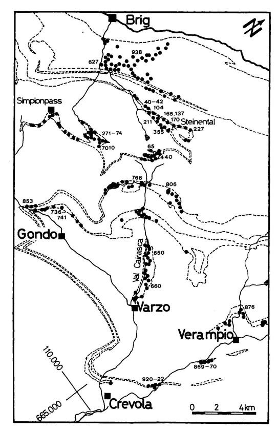
Fig. 2 Outline map of the cross section Brig-Crevola showing principle locations. Countours indicate the regional occurrence of Mesozoic cover rocks, separating the cristalline basement rocks. Sample numbers refer to the specimens which were analyzed by electron microprobe technique.
