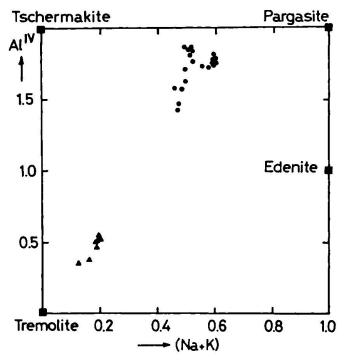
Fig. 19 Compositional variation of Ca-amphibole plotted in a Al<sup>IV</sup>-(Na+K) diagram. Filled circles refer to calcareous rocks, triangles to dolomitic marbles.
