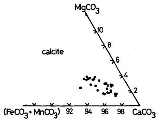
Fig. 26 Calcite composition in terms of MgCO<sub>3</sub>-CaCO<sub>3</sub>-(FeCO<sub>3</sub>+MnCO<sub>3</sub>) components.
