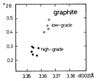
Fig. 25 d(002) spacing values of graphite correlated to the crystallinity index defined as the peak width of d(002) at half peak height. Open circles: graphite from low-grade samples (Brig-Steinental). Filled circles: graphite from high-grade samples (Simplonpass).
