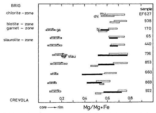
Fig. 31 Variation and change of Mg/Mg+Fe in garnet, staurolite, biotite, chlorite and muscovite along the cross section Brig-Crevola.
