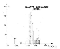
Fig. 11 Distribution of homogeneization temperatures (T°h) of fluid inclusions of quartz crystals, coeval respectively with the beginning (a) of the hydrothermal remobilization of pyrite and (b and c) of the crystallization of haematite.
