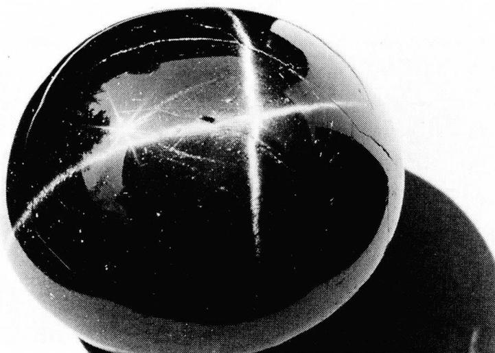
Figure 1 A cut *en cabochon* star diopside from Namakkal (S. India), diameter about 15 mm and weight about 4 g, showing the four-rayed asterism. Note that the arms of the rays do not cross at right angles.
