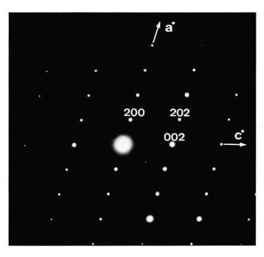
Figure 4 [010] electron diffractogram of diopside.
