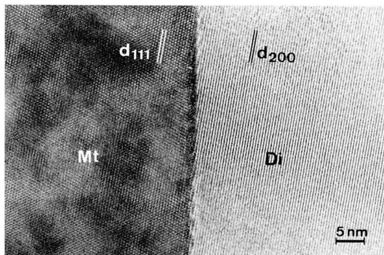
Figure 9 Detail of the intergrowth of a magnetite inclusion and the diopside host. The lattice fringes  $d_{200}$  of diopside are parallel to the  $d_{111}$  fringes of magnetite, which is characteristic for the “Z” type inclusions. The magnetite blades are bounded by irrational planes.
