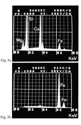
Figure 3 X-ray microanalysis of diopside (a) and a bladeshaped inclusion (b). Only Fe is present as major element in the inclusion.
