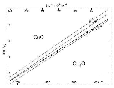
Fig. 2: Equilibrium Cu-Cu<sub>2</sub>O. Abbreviations as in fig. I. H = curve based on equation given by HUEBNER (1971).
