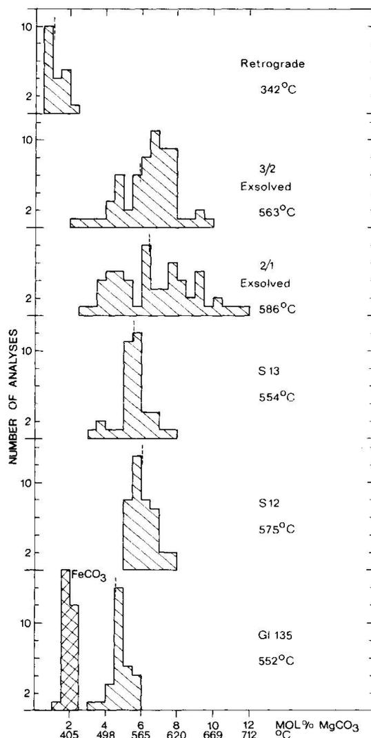
Fig. 6 Histograms of the  $\text{MgCO}_3$ - (and  $\text{FeCO}_3$ )-content of calcites coexisting with dolomite. Gl 135, S 12 and S 13 represent single samples, 2/1 and 3/2 represent single grains and retrograde calcites represent various samples.
