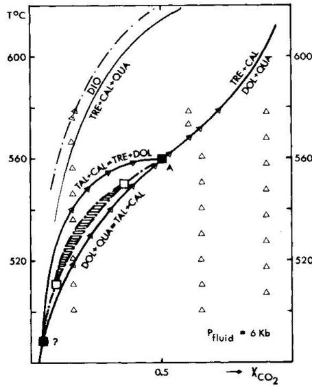
Fig. 9 T- $X_{CO_2}$ -topology derived from the field and calcite-dolomite-geothermometry (see text.) Oblique hatched: stability field of talc and calcite in FeO-bearing metacarbonate G1 135. Arrows indicate path of progressive metamorphism.
