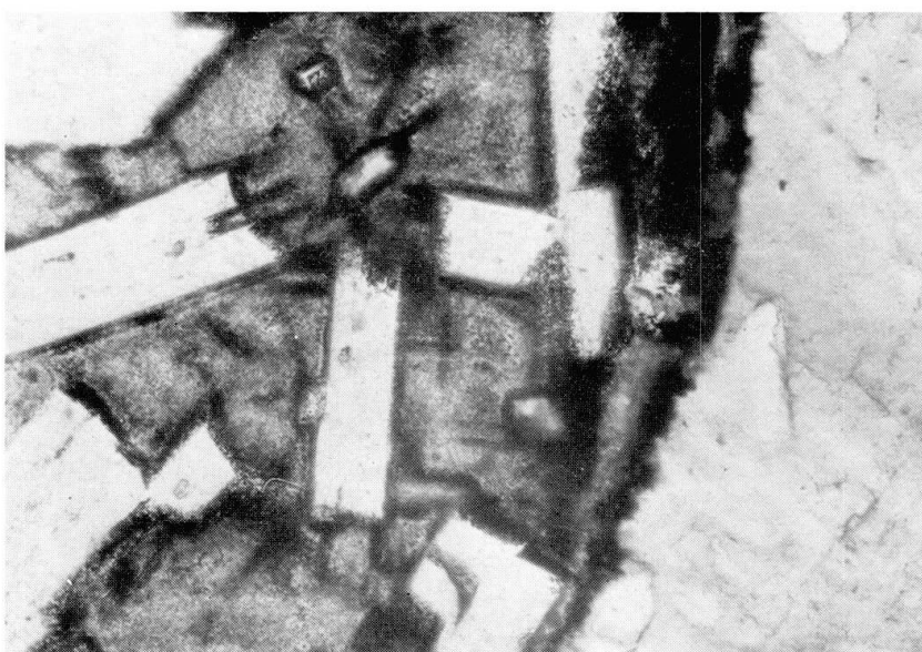
Fig. 7 1 st generation albitite forms euhedral tabular crystals, the interspaces are filled by 2 nd generation anhedral albites. L = 1.30 mm, without analyser)
