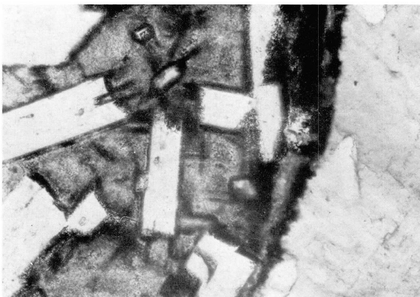
Fig. 7 1 st generation albite forms euhedral tabular crystals, the interspaces are filled by 2 nd generation anhedral albites. L = 1.30 mm, without analyser)
