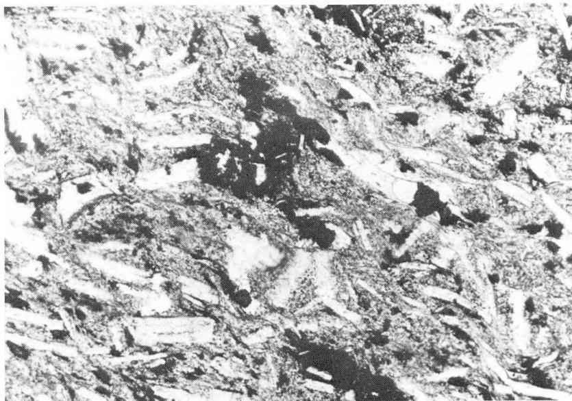
Fig. 4 Chlorite spilite. Euhedral albites with intersertal chlorite and opaques.
