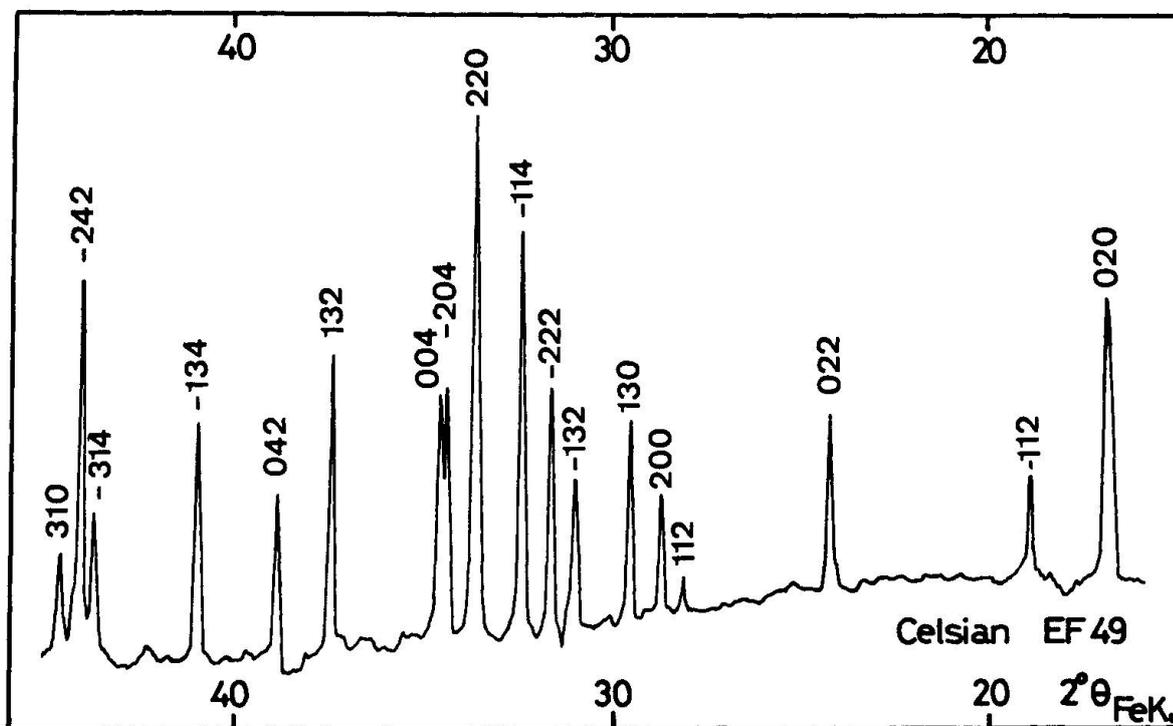
Fig. 2 Recorded intensities of celsian EF 49 (Guinier-film), using a double-beam microdensitometer.
