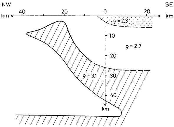
Fig. 2 Model of the crust in the Ivrea Zone region according to the German Research Groupe for Explosion Seismology (BERCKHEMER, 1968).
