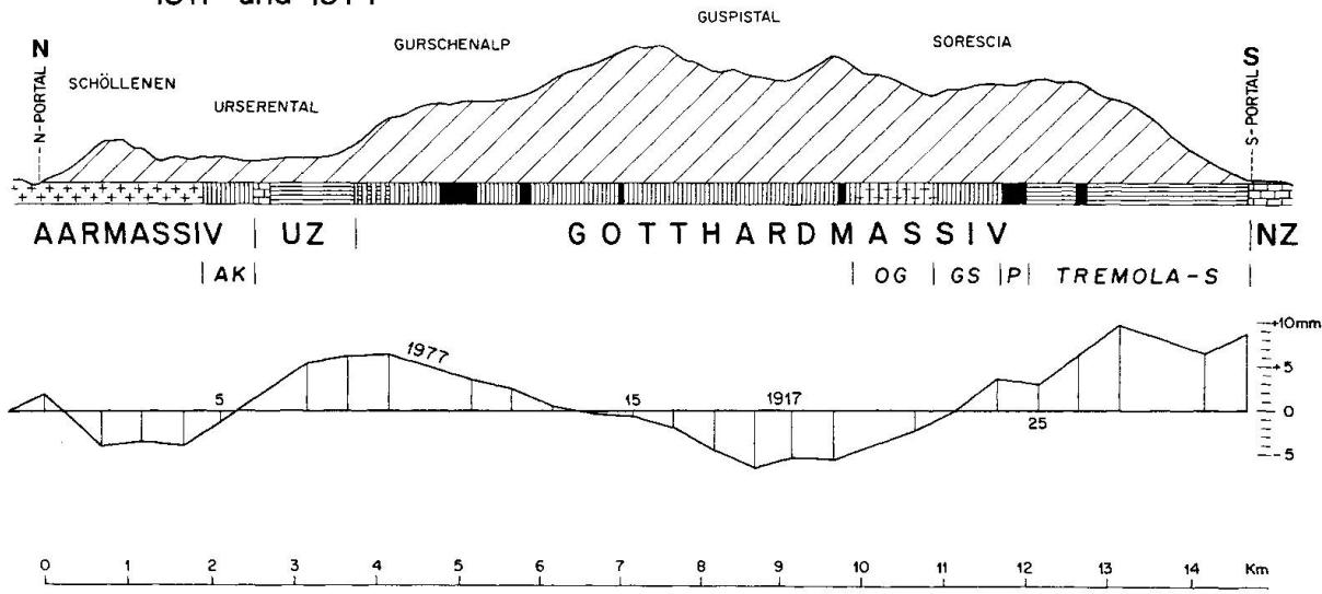
Fig. 4 Gotthard railway tunnel. Height changes of the bench marks between 1917 and 1977 (lower profile), and simplified geological profile. After FUNK & GUBLER, 1979.
