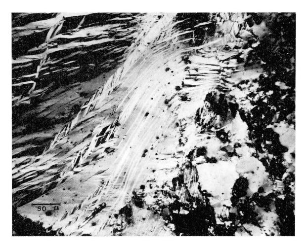
Fig. 5. Stibnite from Su Suergiu mine, deformed according to the open folds of the late tectonic phases. It shows undulatory extinction and twin-gliding parallel to the axial plane of the fold. Polished section, +N.
