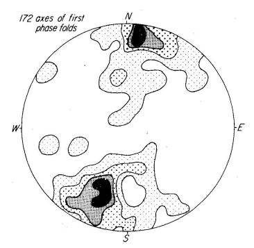
Fig. 2. Statistical diagram of the First phase axes and of the S<sub>0</sub>/S<sub>1</sub> intersection lineations. 1%, 3%, 5%, 7% for 1% of the surface. The variability of the strikes between N 10° W and N 50° E is mainly due to the original dispersion of the First phase axes within their own axial planes. The great variability of the dips is due to the Second phase, striking on the average N 120°, which refolds the linear elements of the First phase.
