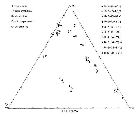
Fig. 5. (Mn)-(Ca)-(Mg+Fe) mol per cent plot of carbonates, rhodonites pyroxmangites, elino-pyroxenes and tephroites of manganese protores samples from Buritirama, analyzed by microprobe. The different coexisting phases are plotted with the same graphical symbols.
