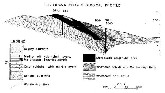
Fig. 3. Geological profile, 200 N of the Buritirama, B-5 orebody after Anderson, Dyer and Torres (1974).
