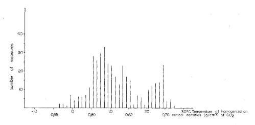
Fig. 6. Critical densities (g/cm³) of CO<sub>2</sub> and temperature of homogenization of 394 fluid inclusions in quartz crystals from Buritirama (B-5-10) braunite marble manganese protore. The quartz occurs in small aggregates associated with different manganese minerals.
