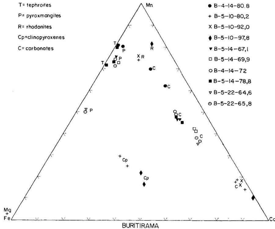
Fig. 5. (Mn)-(Ca)-(Mg+Fe) mol per cent plot of carbonates, rhodonites pyroxmangites, clinopyroxenes and tephroites of manganese protore samples from Buritirama, analyzed by microprobe. The different coexisting phases are plotted with the same graphical symbols.
