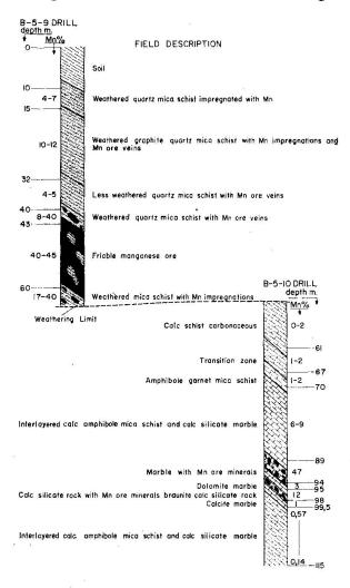
Fig. 4. Schematic lithologic profile of the weathered zone of the B-5-9 diamond drill hole and of the fresh rocks of the B-5-10 diamond drill hole. These drills are located on the Fig. 2 and represented in less detail in Fig. 3. Constructed on the basis description of geologists of Cia Meridional de Mineração and controlled by petrographic and mineralogical studies.
