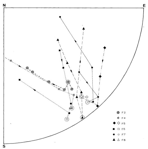
Fig. 3. Stereographic projection of magnetization directions for six dikes during AF cleaning. Solid symbols: lower hemisphere; open symbols: upper hemisphere. The arrows point to increasing  $\mathbf{H}_{\text{peak}}$  field of demagnetization. The large circles enclose the best clustered mean directions.
