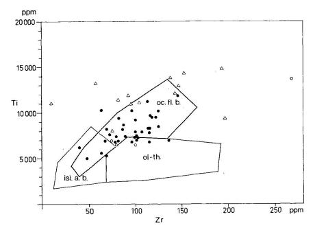
Fig. 8. Ti-Zr diagram (Pearce and Cann, 1973) of the metabasites. Dots represent prasmites and garnet amphibolites of the Dorfer Valley, triangles garnet amphibolites of the Umbal Valley, circles eclogites.
