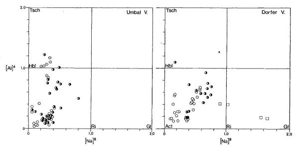
Fig. 12. Compositions of the amphiboles in [Al]<sup>4</sup> versus [Na]<sup>8</sup> diagrams. Symbols as described in Fig. 4; open squares represent alkali amphiboles of the glaucophane schists.
