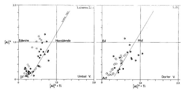
Fig. 10. Compositions of the amphiboles in [Al]<sup>4</sup> versus [Al]<sup>6</sup>+Ti diagrams. Open circles represent amphiboles of the prasinites, half filled circles amphiboles of the garnet amphibolites, centered circles relic amphibole in prasinite.
