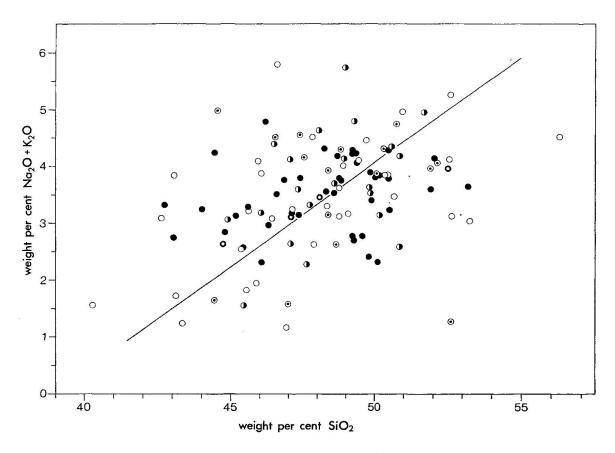
Fig. 5. Representation of the metabasites in a  $Na_2O+K_2O$  versus  $SiO_2$  diagram according to McDonald and Katsura (1964). Solid circles represent prasinites, half filled circles garnet amphibolites, and open circles eclogitic rocks of the Dorfer Valley, centered circles garnet amphibolites of the Umbal Valley.
