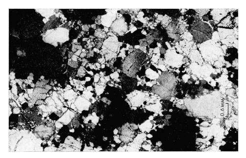
Fig. 3. The chlorite peridotite AR 29, strained olivine porphyroclasts embedded in recrystallized matrix grains. The slightly folded layering  $S_{01}$  is difficult to recognize in this part of the thin section.
