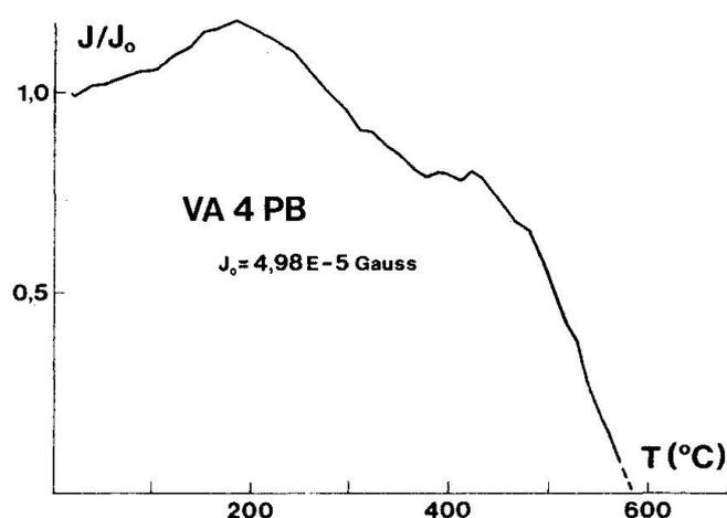
Fig. 3. Continuous thermal demagnetization of AF-cleaned stable NRM.
