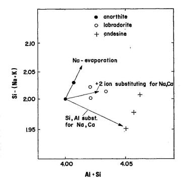
Fig. 5. Variation of Si-(Na+K) and Al+Si in 746b<sub>2</sub> intergrowth. Microprobe analyses of Si, Al, Ca, Na, K normalized to 8 0. Some substitution vectors are indicated. Their length corresponds to 0.05 formula units (compare Wenk and Wilde, 1973).
