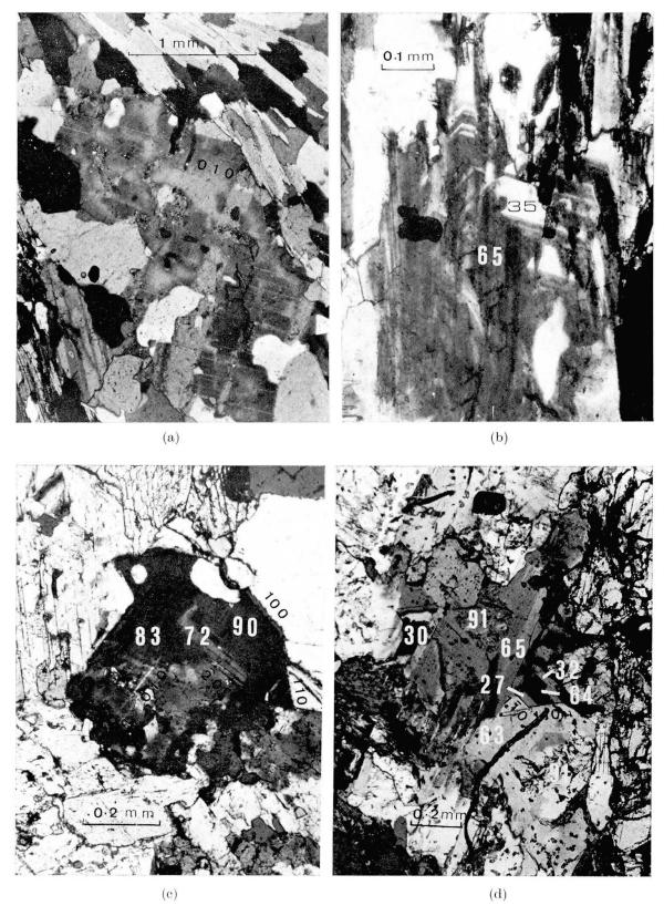
Fig. 4. Photomicrographs of plagioclase intergrowths. Composition is indicated, see Table 1, Miller symbols in black. (a) Andesine An 29–38 with oligoclase An 21–27 inclusions, sample Vz. 594f. (b) Buttress-like labradorite An 62–67-andesine An 31–37 intergrowth, sample Vz. 593d. (c) Inhomogeneous two-bytownite intergrowth, sample Vz. 699. (d) Anorthite, labradorite and andesine, sample Vz. 746b<sub>2</sub>.
