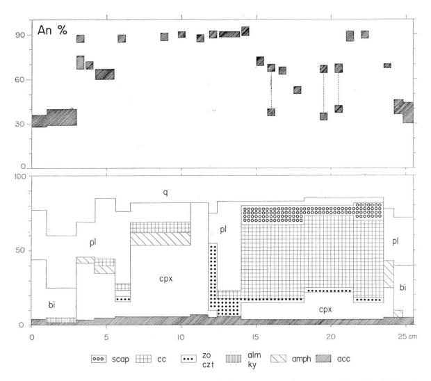
Fig. 2. Variation of plagioclase composition and of mode across the 25.5 cm long banded rock sample Vz. 746 m, examined in seven thin sections cut perpendicular to the foliation. Outcrop Carecchio in main river on northern shore, coordinates 712.25/123.93. Intergrowth of labradorite and andesine is marked by dotted line. Anorthites found in scapolite-marble concern grains surrounded by calcite, diopside and clinozoisite. As accessory mineral sphene is more common than ore minerals.
