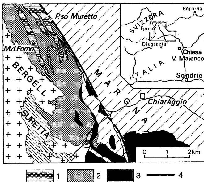
Fig. 1. Geological sketch map of Monte del Forno-Monte Disgrazia area. Metaophiolites and their metasedimentary cover: (1) Diopsidite-plagioclase quartzschists + Andalusite-garnet biotitic schists + Basal Quartzites; (2) Monte del Forno Amphibolites; (3) Malenco Serpentinites; (4) Muretto-Ventina Line.
