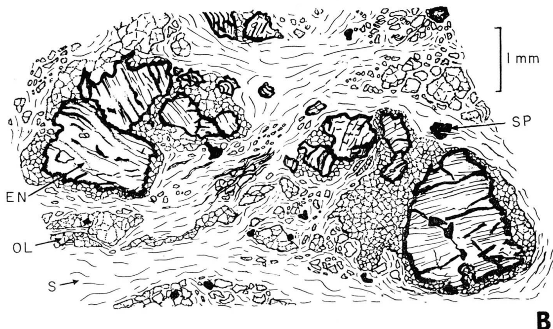
Fig. 2b. Blastomylonitic texture of the harzburgite at Vimy Ridge as seen under the microscope. The porphyroclasts of enstatite are bent and show deformation lamellae; the olivine grains are fractured and granulated and partly serpentized (OL, olivine; EN, enstatite; S, serpentine; SP, spinel).
