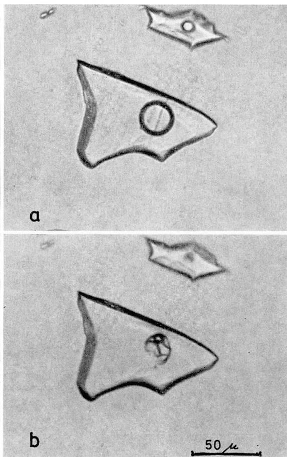
Fig. 6. Fluid inclusions with  $\text{H}_2\text{O-NaCl-CH}_4$ , secondary inclusions: a)  $+25^{\circ}\text{C}$ , bubble of supercritical  $\text{CH}_4$  in water, b)  $-100^{\circ}\text{C}$ , bubble of  $\text{CH}_4$ -gas in liquid  $\text{CH}_4$  surrounded by ice. (Homogenization temperature of  $\text{CH}_4$   $-93^{\circ}\text{C}$ ; Melting point of ice  $-1,5^{\circ}\text{C}$ .)
