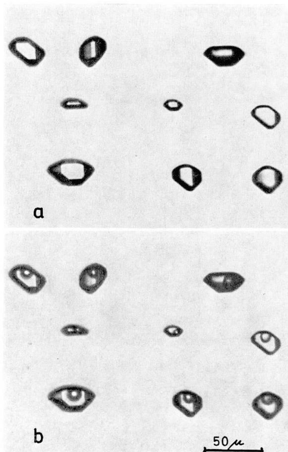
Fig. 5. Fluid inclusions of methane, primary inclusions: a)  $+25^{\circ}\text{C}$ , supercritical state, b)  $-100^{\circ}\text{C}$ ,  $\text{CH}_4$ -gas (bubbles) in liquid  $\text{CH}_4$ . (Homogenization temperature of  $\text{CH}_4$   $-95^{\circ}\text{C}$ .)
