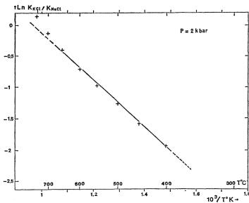
Fig. a 2. Variations of the ratio of conventional dissociation constants of KCl and NaCl with temperature at 2 kbar total pressure.
