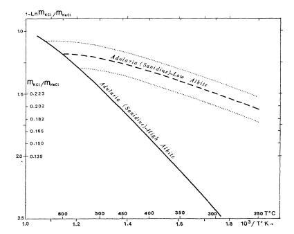
Fig. 6. K/Na atomic ratio in solutions at equilibrium with two alkali feldspars, as a function of temperature. The curves are probably valid in the 1–3 kbar pressure range.
