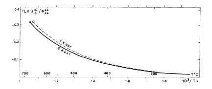
Fig. a 4. Negative logarithm of the ratio of activities of orthoclase and albite in coexisting alkali feldspars as a fonction of temperature, at 1 and 2 kbar.
