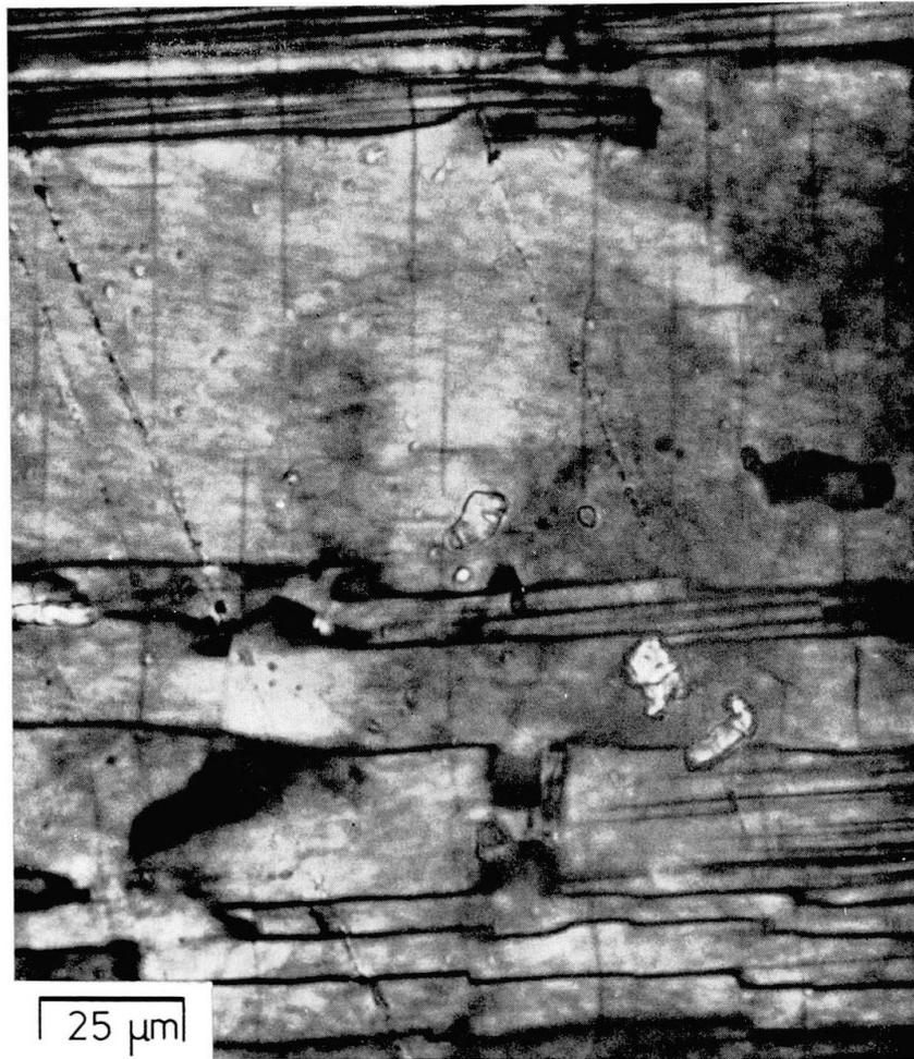
Fig. 2. 1000 kV electron micrograph showing elongated subgrains approximately parallel to exsolution lamellae.
