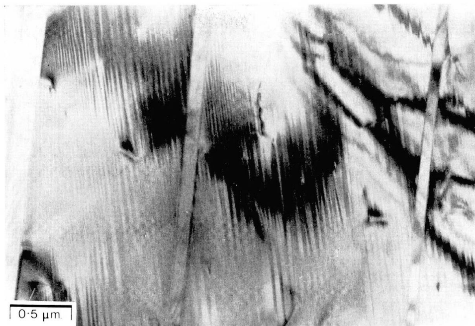
Fig. 5. 100 kV electron micrograph showing the variation in periodicity of the exsolution lamellae and three Albite twins (approximately vertical). The wavelength of the exsolution varies from 20 to 80 nm.
