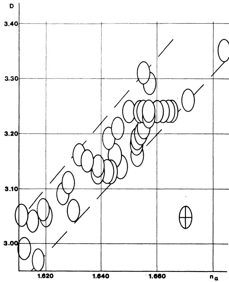
Fig. 13. Density vs n of calcic amphiboles.
