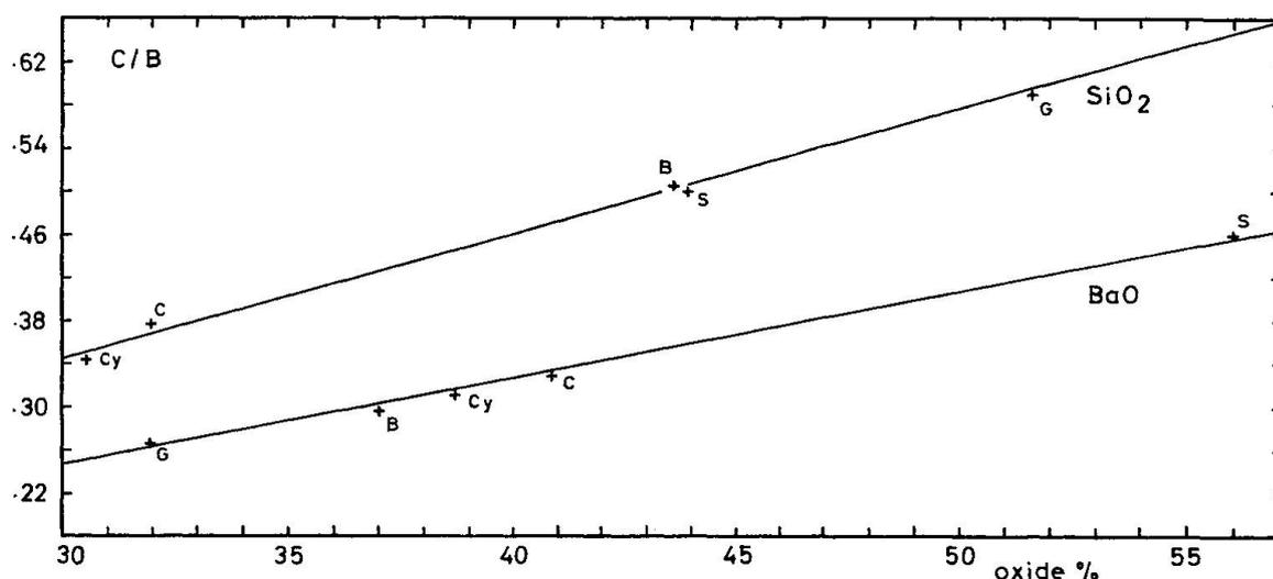
Fig. 1. Working curves for BaO and SiO<sub>2</sub>. Plot of counts/beam current (C/B) vs. oxide weight percent of standards. C: celsian, Cy: cymrite, B: benitoite, G: gillespite, S: sanbornite.
