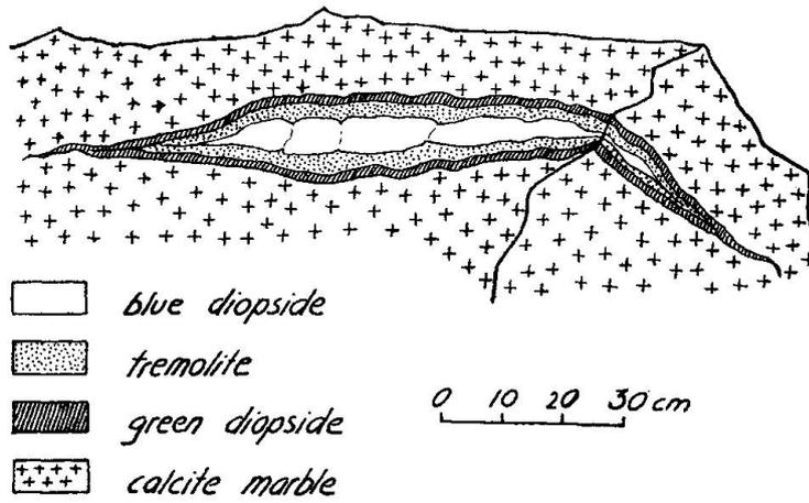
Fig. 1. Schematic sketch of the lens of blue diopside in Val Sissone.
