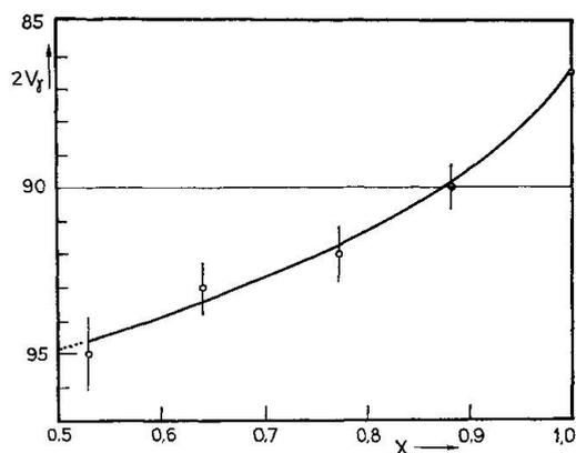
Fig. 3. Optic axial angle of mixed crystals  $(\text{NH}_4)_x\text{K}_{x-1}\text{NO}_3$ . The vertical lines represent the dispersion of the determinations made for each concentration (about 10) (see LEONE, 1970).
