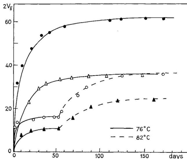
The intermediate phase II' is obtained by annealing crystals of II in the stability range of III. Crystals of tetragonal or lower symmetry are obtained. After a certain length of time the crystals turn biaxial by annealing.  $2V_{\gamma}$
