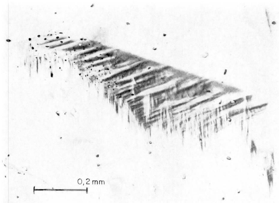
Fig. 5. Tridymite lamellae in quartz. Crossed polars. The lamellae form with each other an angle of  $\pm 106^\circ$ . The axial angle of the material of the lamellae is  $2V_z = 36^\circ$ . The acute bisectrix coincides with the optical axis of the surrounding quartz. Stereographic projection Fig. 16.
