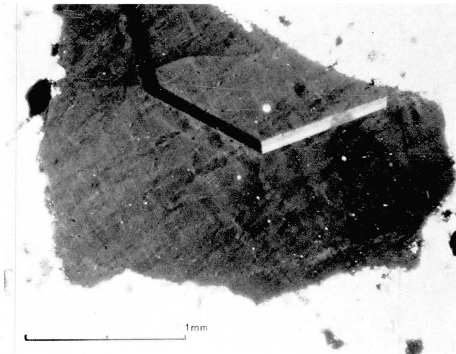
Fig. 9. Frame-like interposition of tridymite in quartz. Crossed polars. U-stage determinations show that the three laths (length  $\sim 0.7$  mm, width  $\sim 0.08$  mm) are biaxial and that their acute bisectrices coincide with the optical axis of the surrounding quartz. Stereographic projection Fig. 17. In the lath at right, there is a different orientation on the two parts of the lath separated by the median line, parallel to the elongation.
