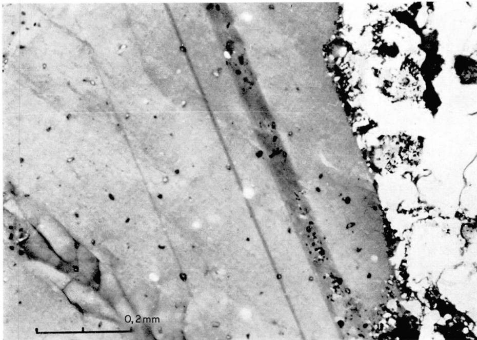
Fig. 8. Tridymite lamellae in quartz. Crossed polars. Aspect resembling that of polysynthetic twinning lamellation. U-stage determination of the broad lamella (width  $\sim 0.03$  mm) shows that the material is biaxial;  $2V_z = 23^\circ.5$ ; the acute bisectrix coincides with the optical axis of the surrounding quartz.
