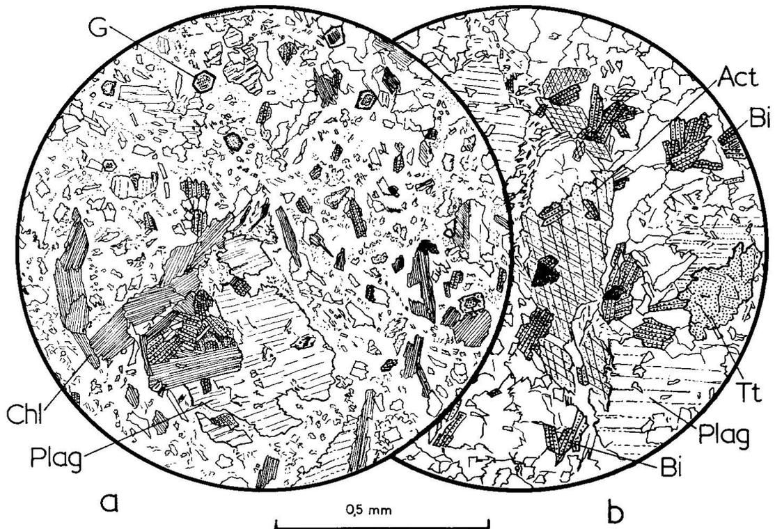
Fig. 11. a, Thin section drawing of garnetiferous hornfels with plagioclase ( $An_{25-30}$ ) porphyroblast, biotite and later chlorite. Idiomorphic. b, meta-psammite from the Pelitic Member with plagioclase, actinolite, biotite and titanite (Tt).
