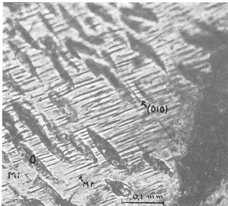
Fig. 4. Ancient oligoclase remnants (O) in the microperthite. Section  $\perp$   $(\bar{6}01)$ ; (010) is somewhat inclined. Constant inclination of the microplagioclase (M.P.) to the cleavage was determined. The distribution of the remnants is rather irregular. Due to the difference of the refractive indices the relief of the unmixed oligoclase against microcline (Mi) is visible (sample 55).
