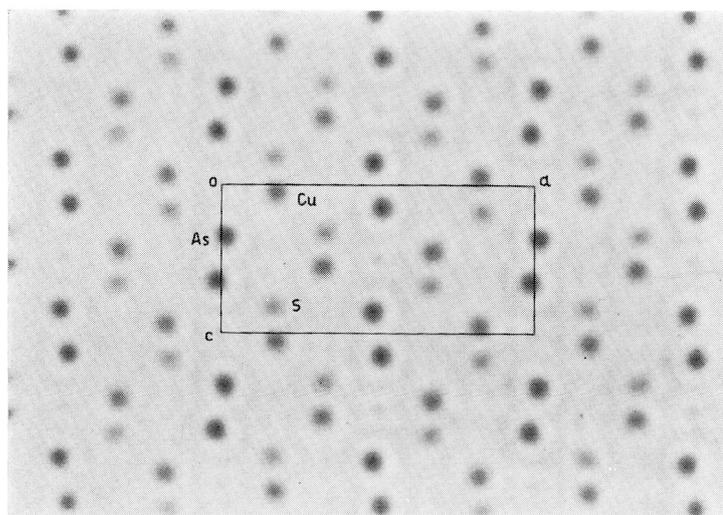
Fig. 4. Electron density projection along the  $b$ -axis.Table 2. *Observed and calculated structure amplitudes*
