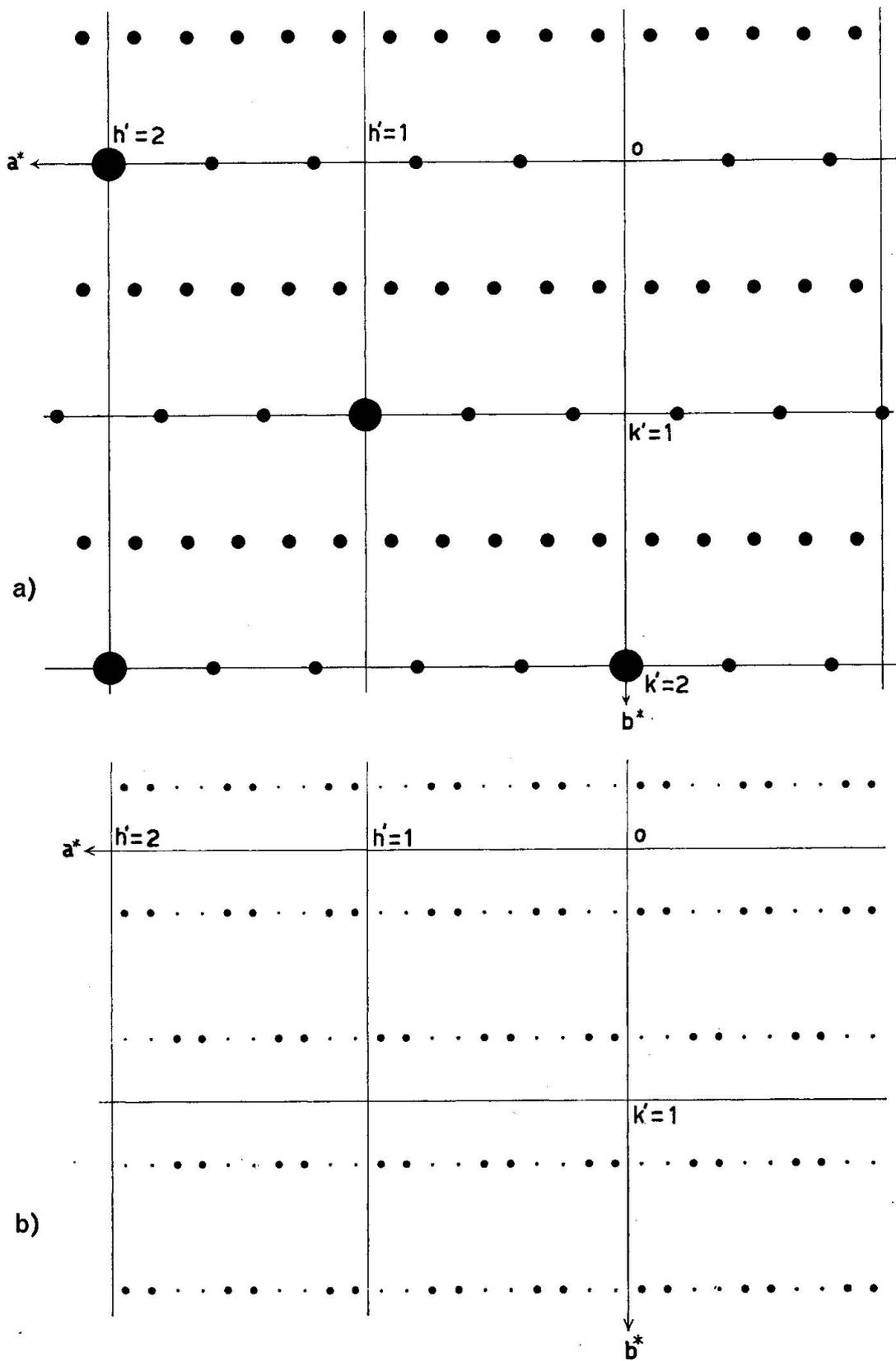
Fig. 6. The reciprocal lattice of sinnerite, a)  $(h, k, 4n)$ , b)  $(h, k, 4n + 1)$ , c)  $(h, k, 4n + 2)$  and d)  $(h, k, 4n + 3)$ , where  $n = \text{integer}$ . The reciprocal lattice points are classified
