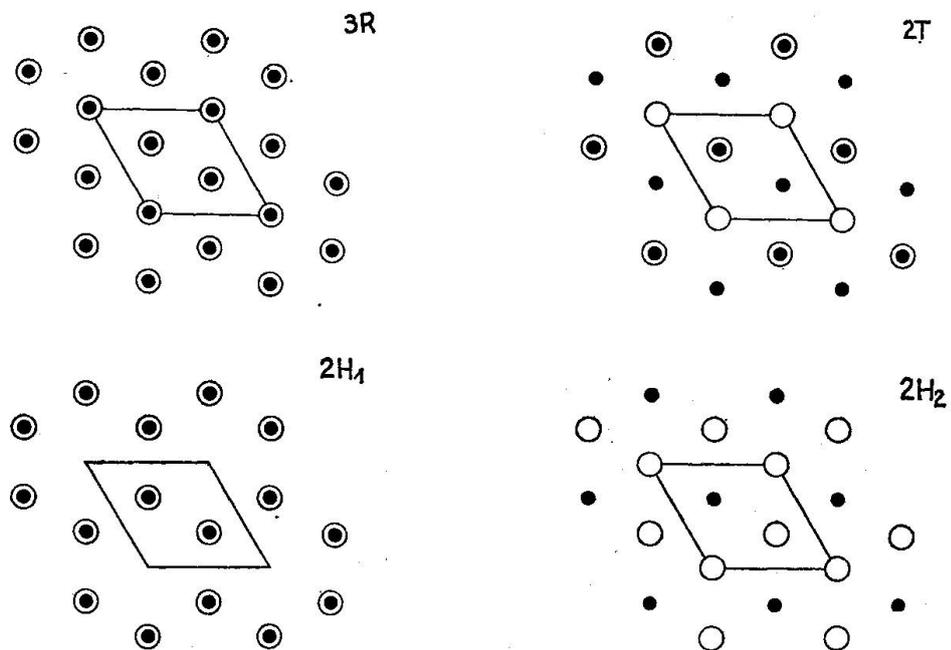
Fig. 5. Structures of simple polytypes projected along the  $c$ -axis. The origin of  $2H_2$  is not taken on a six-fold screw axis. To compare with Fig. 6, the origin of  $2H_2$  should be shifted to  $(\frac{2}{3}, \frac{1}{3}, 0)$  and that of  $2T$  to  $(\frac{1}{3}, \frac{2}{3}, 0)$ . ( $\bullet = \text{Mo}$ ,  $\circ = \text{S}$ ).
