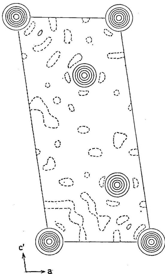
Fig. 3. Final Fourier projection of rhombohedral  $MoS_2$ . Contours are drawn at intervals of  $10 \text{ e} \cdot \text{A}^{-2}$  for S and  $30 \text{ e} \cdot \text{A}^{-2}$  for Mo, starting from  $10 \text{ e} \cdot \text{A}^{-2}$ . Zero contours are shown by broken lines.
