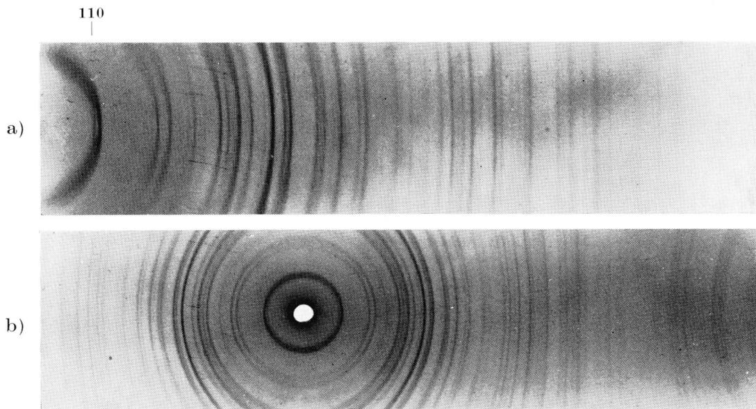
Fig. 1. Ferrian sodium-amphibole from Vals. Co  $K\alpha$  radiation.
