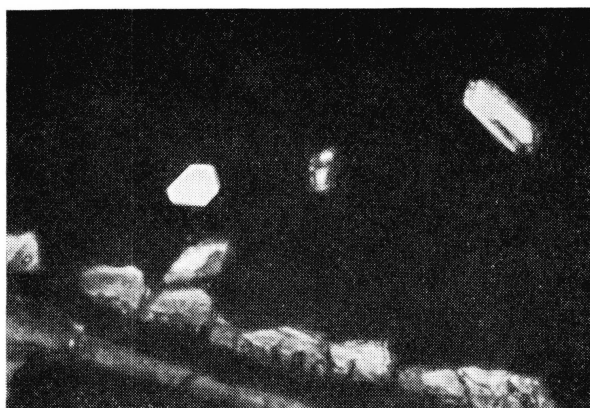
Fig. 1. Photomicrograph of strychnine crystals lying on a glass carrier. Crossed Nicols, 42.5\times .
