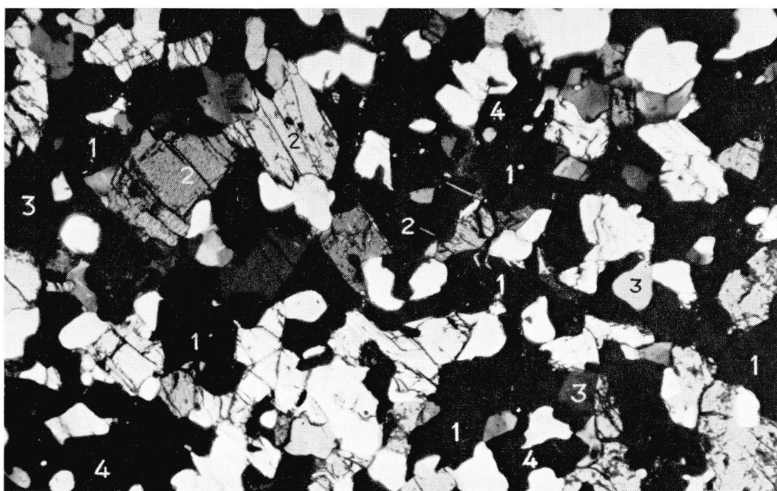
Fig. 2. Amphibolite containing isotropic unknown mineral N of Belihun, Sierra Leone. Thin section 40\times . N + . 1 = dixeyite; 2 = hornblende; 3 = quartz; 4 = magnetite.
