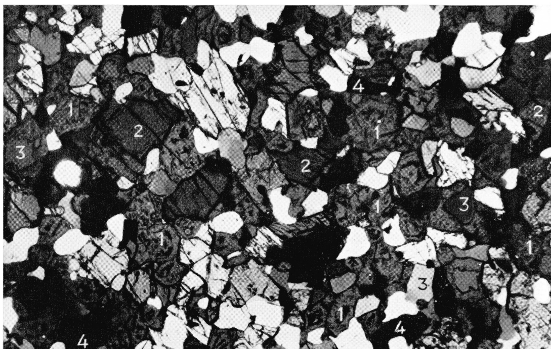
Fig. 1. Amphibolite containing isotropic unknown mineral N of Belihun, Sierra Leone. Thin section 40\times . N // . 1 = dixeyite; 2 = hornblende; 3 = quartz; 4 = magnetite.
