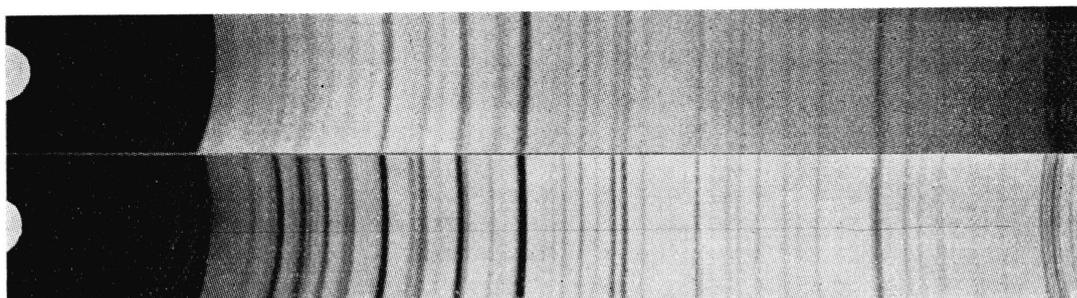
Fig. 2. X-ray powder photographs (Cu-radiation); bottom: standard quartz photograph, top: Pumphrey Mt. Specimen.
