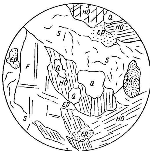
Fig. 5. The same rock (Pe 33) showing formation of garnet at the contact; feldspar also saussuritised
