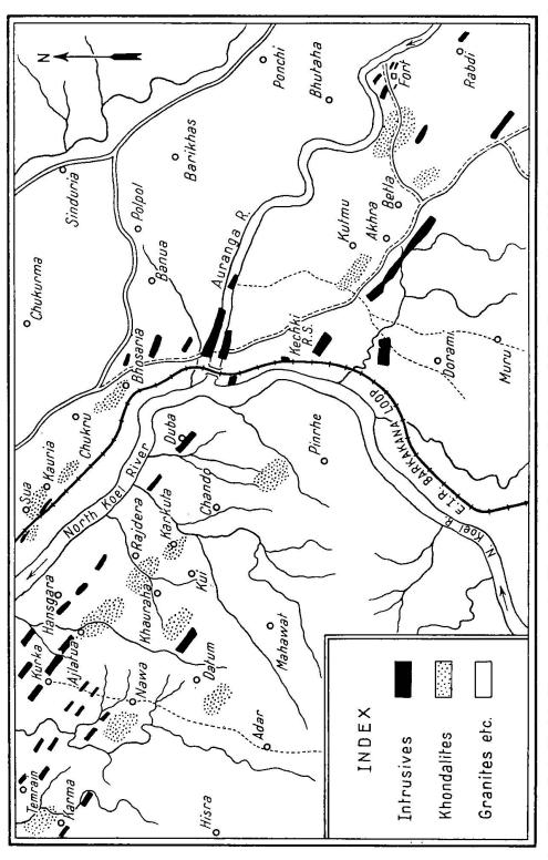
= 2 miles = 3.2 km, of the Auranga-Koel Valley, Palamau district, showing the distribution of khondilites (dotted) and basic intrusives (thick lines and dashes) within granites and gneisses (without signature) forming the basement of the whole area. Pegmatites and aplites occuring in swarms in the area are not shown Fig. 1. Geological Sketch Map on scale 1"
