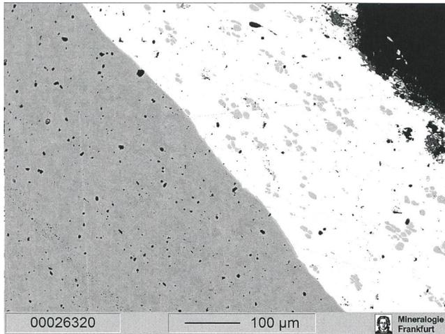
**Figure 6: Coin 4. Backscattered image (BSE), electron microprobe analysis: Wavy surface of the iron flan (left, BSE: grey) indicating the flattening process. Right in the image is the copper layer (BSE: white; coin is diagonally oriented). Upper right corner (black) is resin.**
