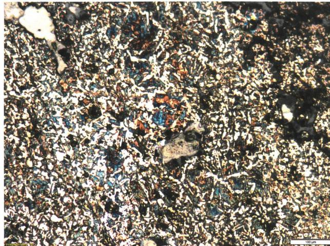
Figure 8: Iron flan of coin 4 as etched with Nital. View towards the edge of the coin, where needle-like ferrite-perlite structure developed, which forms when hypo-eutectic Fe-C with < 0.8 % C was overheated (magnification = 20 ×).
