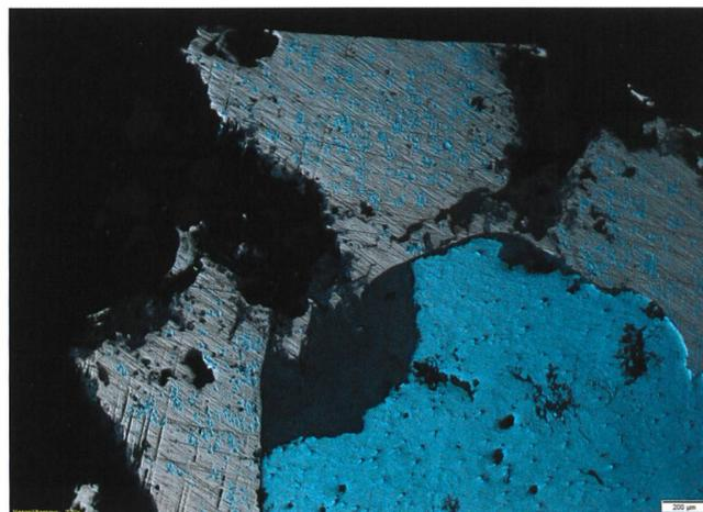
**Figure 11: Coin 4.** One of the two barrel-shaped edges of coin 4. The iron flan is significantly dented and the barrel shape is distorted. Where the copper sheet has broken apart, the iron flan is weakened and in consequence heavily corroded. The copper layer appears as cut surfaces.
