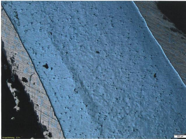
**Figure 9: Polarized microscope, cross polished section of the subferrate coin 4 as polished. Core (blue) = iron flan, layer (brown/blue) = copper layer. The thickness of the copper layer is 300–350  $\mu\text{m}$ .**
