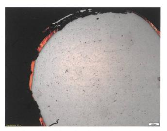
Figure 16: Barrel shape of iron flan from the experiment.
