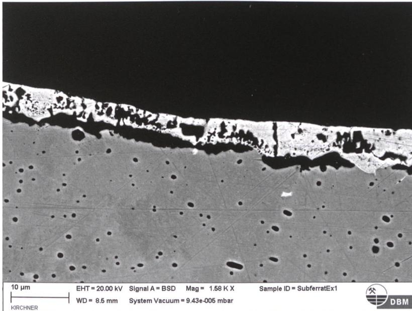
**Figure 19:** Backscattered electron image of the experiment. Porosity weakens the adherence between the copper layer and the iron flange.
