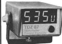
Tachometer TT 84 / TDZ 87 Spraycontrol HT85
