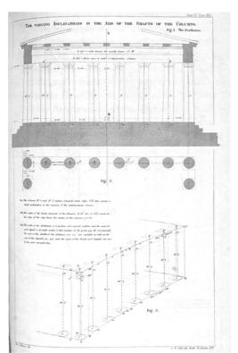
Abb. 6: "The varying Inclinations in the Axis of the Shafts of the Columns. Fig. 1 The Parthenon.", Lithographie gez. von John Robinson, lith. von F. Kell, in: John Pennethorne, Esq., The Geometry and Optics of Ancient Architecture. Illustrated by Examples from Thebes Athens and Rome. Assisted in the Drawing and Colouring of the Plates and in the Arrangement of the Text by John Robinson. Architect, London and Edinburgh: Williams and Norgate 1878, Teil IV, Plate XVI
