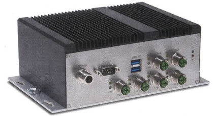
AI Vehicle Computer RM A2 Jetson TX.
