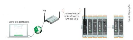
**Figure 6** Smart energy management system Sems.
