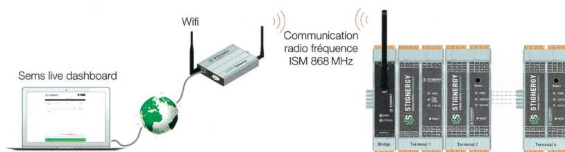
Figure 6 Smart energy management system Sems.
