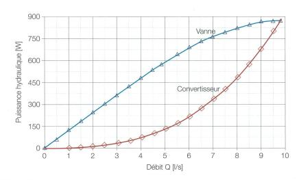
Figure 4 Puissances hydrauliques fournies.
