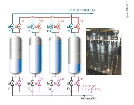
Figure 6 Pressure Swing Adsorption.
