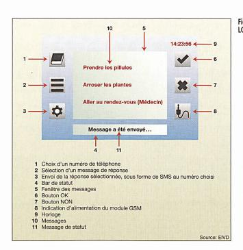
Figure 4 Interface sur LCD [3] B.A. Wilson et al.: Reducing everyday memory and planning problems by means of a paging system: a randomised control crossover study, Jour-
