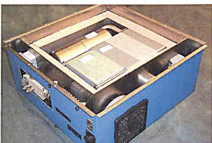
SOFC Auxiliary Power Unit (APU/Quelle: Delphi).
