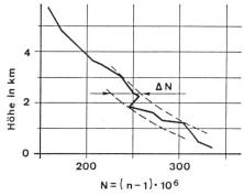
$\begin{array}{ll} {\bf Figur~F1} & {\bf M\"{o}gliches~H\"{o}henprofil~des} \\ {\bf Brechwertes~} N \end{array}$
