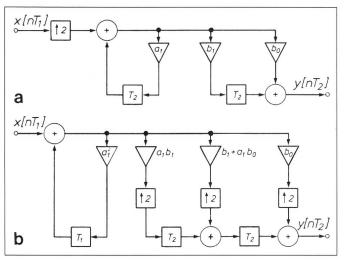
Figur 50. Interpolationsfilter
