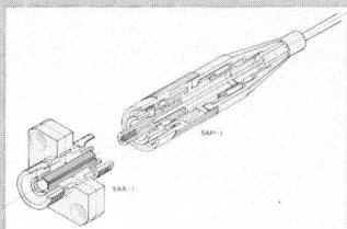
Electronics substantially reduced. The insertion losses are typically 0.4 dB (50/125 GI normal mode) and 1 dB (10/125 SM).
