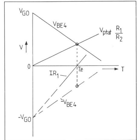
Fig. 10 Calibration of the temperature sensor from figure 9
