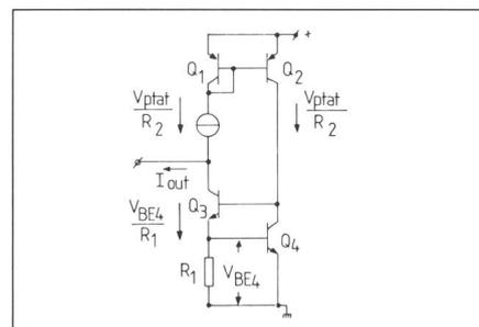
Fig. 9 Intrinsically referenced current source [5]
