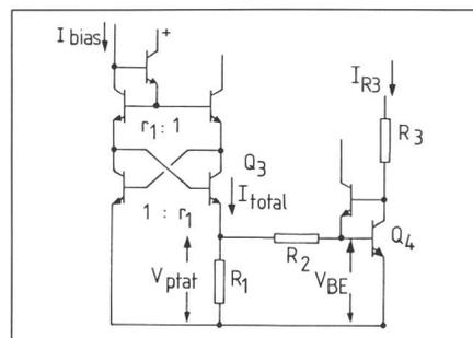
Fig. 14 Temperature-to-current converter
