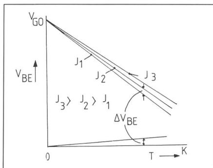
Fig. 3  $V_{BE}$  and  $\Delta V_{BE}$  for different current densities  $J$  as  $F(T)$
