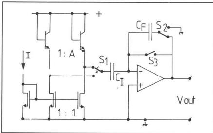
Fig. 11 Switched capacitor approach of a  $V_{PTAT}$  source [8]
