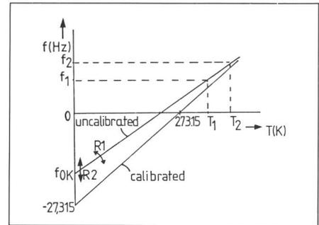
Fig. 15 Calibration of the temperature controlled oscillator
