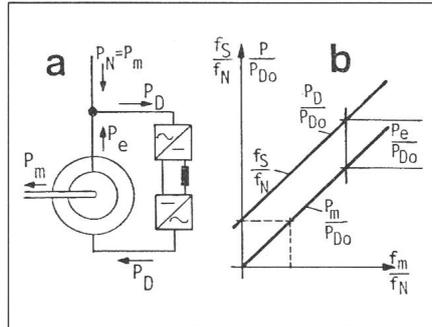
Fig. 8 Schematic diagram and characteristics of a double-fed asynchronous machine
