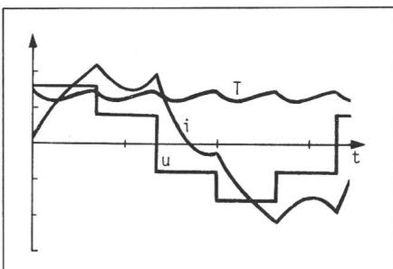
Fig. 3 Voltage, current and torque in a motor fed by a voltage-source inverter (fig. 1b)
