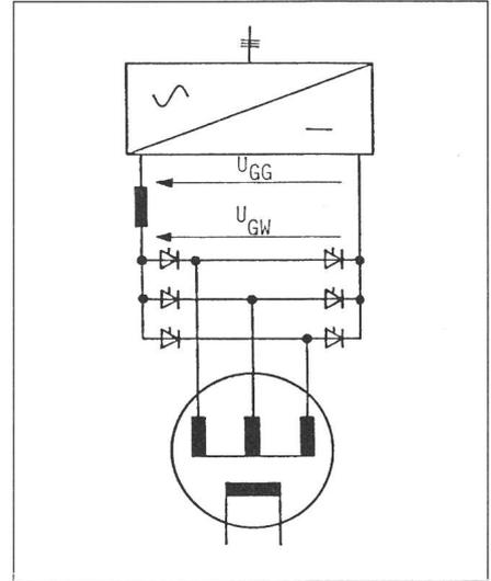
Fig. 5 Synchronous machine fed by a current-source inverter
